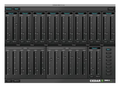
The DNS 8 Live incorporates its remote control software in the form of an internal web page, and you may connect to this using a suitable browser.
