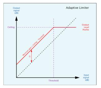
This above illustrates the relationship between the input signal level and the output signal level, and shows how this is affected by the Threshold and Ceiling controls. These can be defined as follows:
